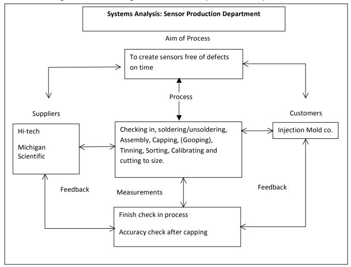
This *System Analysis of the Sensor Department* shows how different parts of the system affect everything that is involved in the final production of a sensor. This tool showed every process that went into the creation of the final product and took the team in the direction of investigating problems involved in each process in the production department. It also showed how the check-in process affects the department as a whole.
