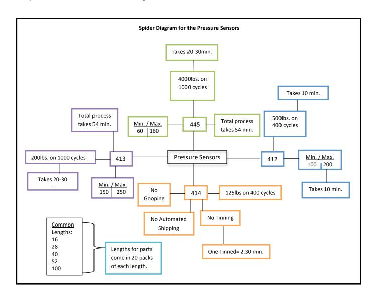
In the *Spider Diagram for The Pressure Sensors* above, the pressure sensors is the main topic to branch off. Then the four different kinds of pressure sensors and their contents were listed. While creating this, tool the team noticed that the 414 sensor was the only one that wasn't automatically shipped, the wire wasn't tinned, and it needed "goop" on it. This lead to more questions on why the other sensors had those features and the 414 did not.
