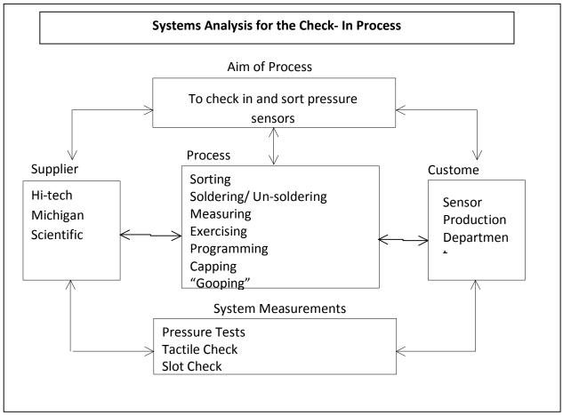
It shows the connection between the overall aims, the customers, the suppliers, and the measurements associated with the Check-In process. This, along with the flow chart, gives a greater understanding of the aspects of the Check-In process.
