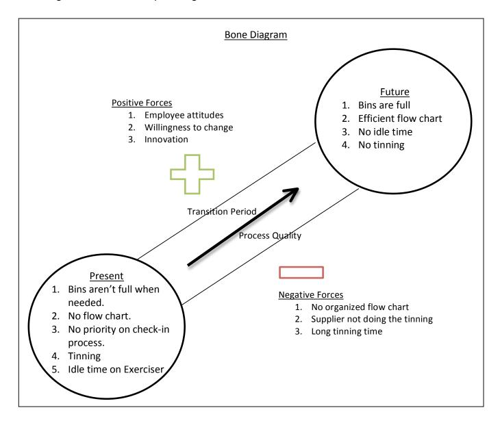
This bone diagram helped the team see the overall process of getting from the present state to the future state. During this process, they found that the tinning on the 414 wire could be done for free by Michigan Scientific. This would eliminate labor time on the 414. Although the team
